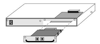
Figure 2-6 Inserting the FE Module Assembly
